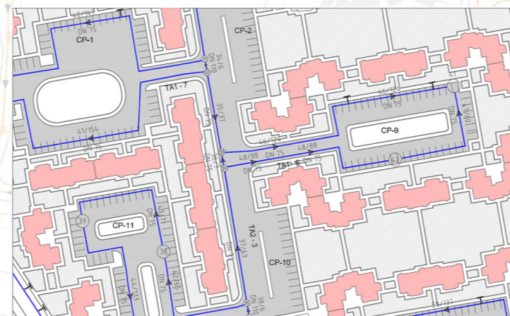
Water Distribution System Model
